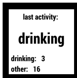
Figure 10: Test app using the logistic regression parameters detecting drinking ADL in real time
