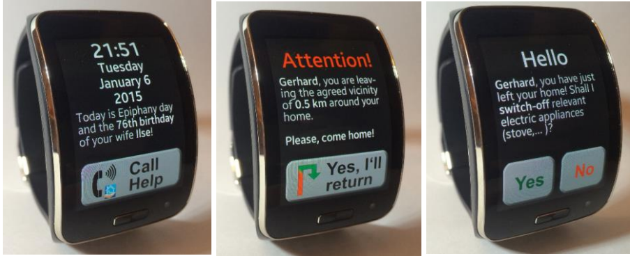
Figure 1: Smartwatch Samsung Gear S running a specialized emergency app, supporting elderly or handicapped persons, e.g. with MCI (mild cognitive impairment) (see [14]).
